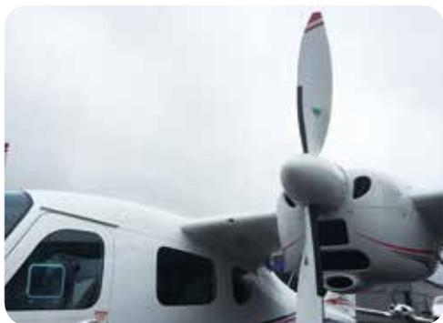
The Rotax 912S and two-bladed propeller.
