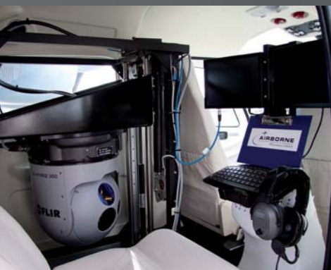
Camera Lift and Sensor Operator Station
