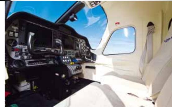
**“**Entering the cockpit is easy as the seats slide rearwards a long way and there is no need to clamber over cockpit equipment
